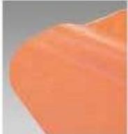
Balloon silk E.g. coated and rubberized fibers; man-made, waterproof materials.
