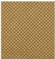
Aramid fiber Kevlar™ Synth. Polyamid-fiber in woven, non-woven, unidirectional form.
